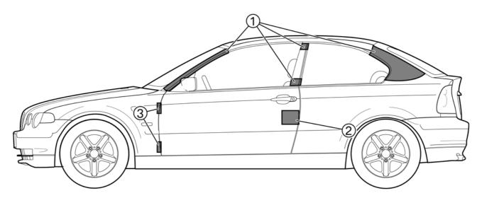
1 The areas mark points at which the roof can be disconnected. Modern high-performance cutters are required for cutting open the bodywork; older hydraulic cutting devices may be insufficient.
